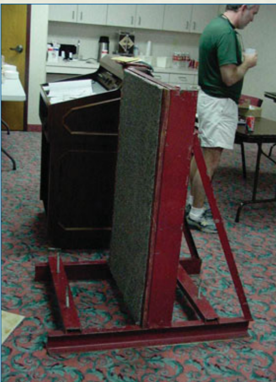
2. Door removal cradle used with Pallet Jack.
